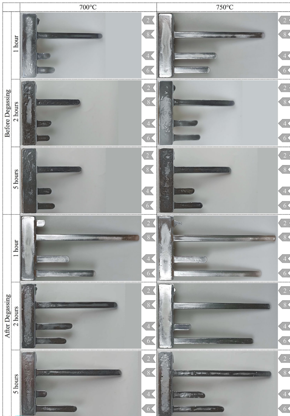
Figure 4. Fluidity test results of carbon steel dipped A356 alloy.
